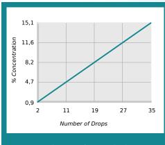
% Concentration = No. of Drops x Titration Factor Titration Factor = 0,43
