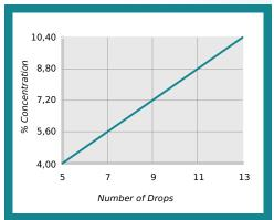
% Concentration = No. of Drops x Titration Factor Titration Factor = 0,80
