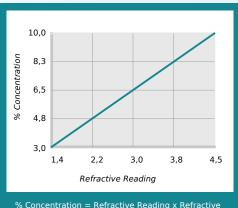
% Concentration = Refractive Reading x Refractive Factor Coolant Refractometer Factor % Brix = 2,2
