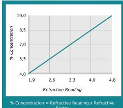
Concentration = Refractive Reading x Refractive Factor Coolant Refractometer Factor % Brix = 2,1
