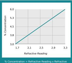
Concentration = Refractive Reading x Refractive Factor Coolant Refractometer Factor % Brix = 1,8
