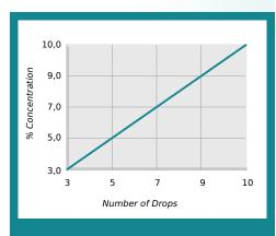
% Concentration = No. of Drops x Titration Factor Titration Factor = 1,00
