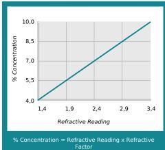
Coolant Refractometer Factor % Brix = 2.9
