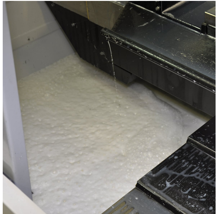
Foam in metalworking fluids can be a necessity or a major headache, with major headache winning out most of the time. Foam doesn't lubricate well, it cools poorly, it increases fluid volume, it adds to odor problems, and most importantly, it can damage machine plumbing.
