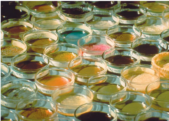
A simple but effective method for checking possible residue effects is to pour 5 ml. of coolant concentrate into a petri dish and leave it exposed to the air at room conditions for a month or more.
