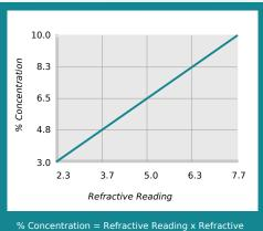
Coolant Refractometer Factor % Brix = 1.3
