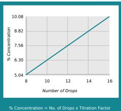
6 Concentration = No. of Drops x Titration Factor Titration Factor = 0.63
