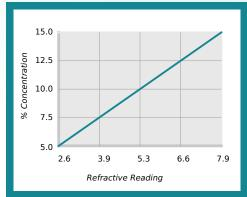
% Concentration = Refractive Reading x Refractive Factor Coolant Refractometer Factor % Brix = 1.9
