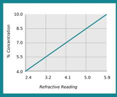
% Concentration = Refractive Reading x Refractive Factor Coolant Refractometer Factor % Brix = 1.7
