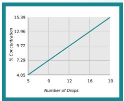
% Concentration = No. of Drops x Titration Factor Titration Factor = 0.81
