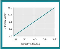
% Concentration = Refractive Reading x Refractive Factor Coolant Refractometer Factor % Brix = 2.2
