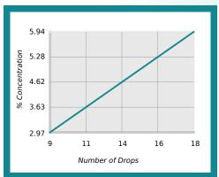
% Concentration = No. of Drops x Titration Factor Titration Factor = 0.33
