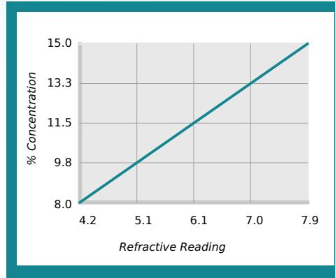
% Concentration = Refractive Reading x Refractive Factor
