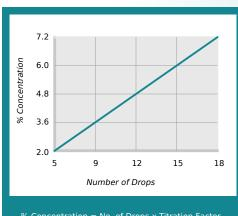
% Concentration = No. of Drops x Titration Factor Titration Factor = 0.40
