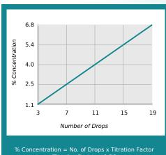
% Concentration = No. of Drops x Titration Factor Titration Factor = 0.36
