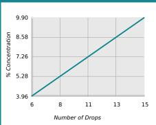
% Concentration = No. of Drops x Titration Factor Titration Factor = 0.66
