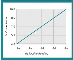
% Concentration = Refractive Reading x Refractive Factor Coolant Refractometer Factor % Brix = 3.3
