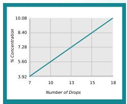
% Concentration = No. of Drops x Titration Factor Titration Factor = 0.56
