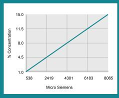
% Concentration = Conductivity in Micro Siemens x Factor Conductivity Factor = 0.00186
