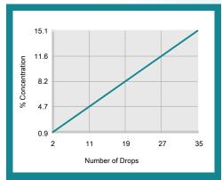
% Concentration = No. of Drops x Titration Factor Titration Factor = 0.43
