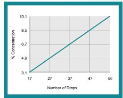
% Concentration = No. of Drops x Titration Factor Titration Factor = 0.18
