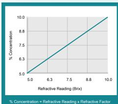
6 Concentration = Refractive Reading x Refractive Factor Coolant Refractometer Factor % Brix = 1.0
