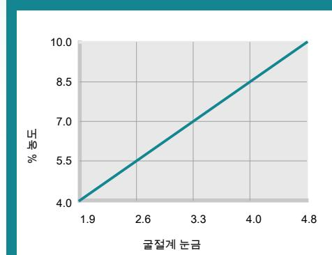
$$\% \text{ 농도} = \text{굴절률} / \text{판독값} \times \text{굴절인수}$$
