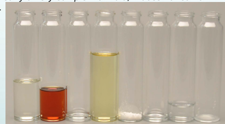
A typical Master Fluid Solutions emulsion concentrate is comprised of 8 ingredients.
