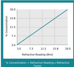
Coolant Refractometer Factor % Brix = 1.0
