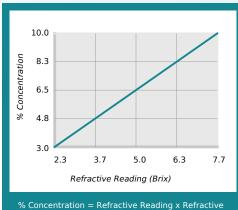
Concentration = Refractive Reading x Refractive Factor Coolant Refractometer Factor % Brix = 1.3
