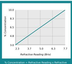
Coolant Refractometer Factor % Brix = 1.3
