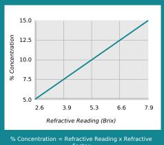
6 Concentration = Refractive Reading x Refractive Factor Coolant Refractometer Factor % Brix = 1.9
