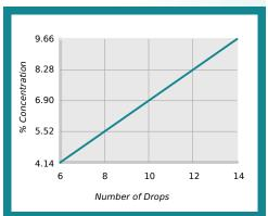
% Concentration = No. of Drops x Titration Factor Titration Factor = 0.69
