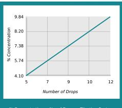
% Concentration = No. of Drops x Titration Factor Titration Factor = 0.82
