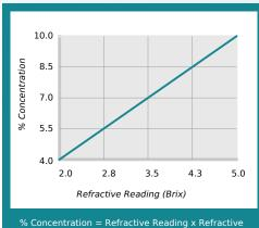
% Concentration = Refractive Reading x Refractive Factor Coolant Refractometer Factor % Brix = 2.0
