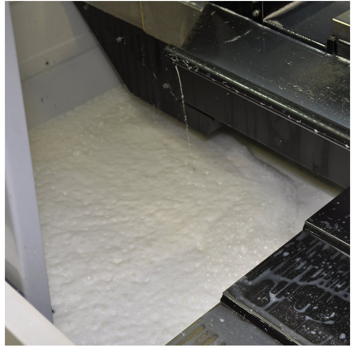
Foam in metalworking fluids can be a necessity or a major headache, with major headache winning out most of the time. Foam doesn't lubricate well, it cools poorly, it increases fluid volume, it adds to odour problems, and most importantly, it can damage machine plumbing.
