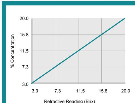
% Concentration = Refractive Reading x Refractive Factor
