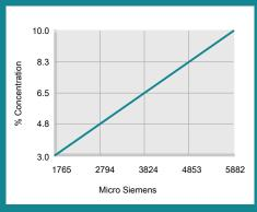
% Concentration = Conductivity in Micro Siemens x Factor Conductivity Factor = 0.00170
