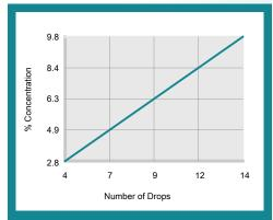
% Concentration = No. of Drops x Titration Factor Titration Factor = 0.70
