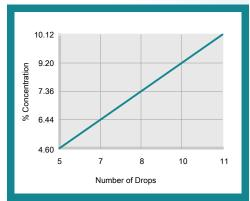
% Concentration = No. of Drops x Titration Factor Titration Factor = 0.92
