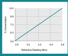
% Concentration = Refractive Reading x Refractive Factor Coolant Refractometer Factor % Brix = 1.8
