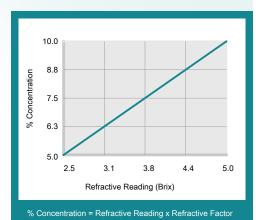
Coolant Refractometer Factor % Brix = 2.0
