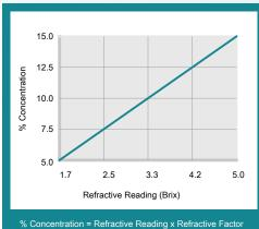
6 Concentration = Refractive Reading x Refractive Factor Coolant Refractometer Factor % Brix = 3.0
