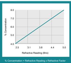
Coolant Refractometer Factor % Brix = 1.6
