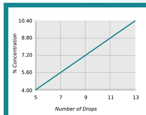
$\% \text{ Concentration} = \text{No. of Drops} \times \text{Titration Factor}$
