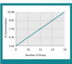
% Concentration = No. of Drops x Titration Factor Titration Factor = 0.63
