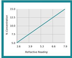
% Concentration = Refractive Reading x Refractive Factor Coolant Refractometer Factor % Brix = 1.9
