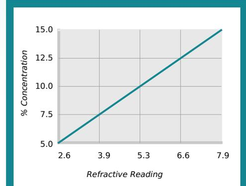
$\% \text{ Concentration} = \text{Refractive Reading} \times \text{Refractive Factor}$
