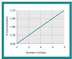
% Concentration = No. of Drops x Titration Factor Titration Factor = 0.42
