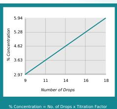
% Concentration = No. of Drops x Titration Factor Titration Factor = 0.33
