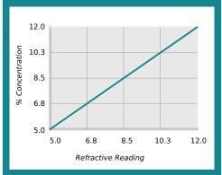
% Concentration = Refractive Reading x Refractive Factor Coolant Refractometer Factor % Brix = 1.0
