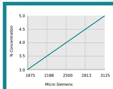
$$\% \text{ Concentration} = \text{Conductivity in Micro Siemens} \times \text{Factor}$$
