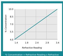
Factor Coolant Refractometer Factor % Brix = 2.9
