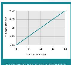
% Concentration = No. of Drops x Titration Factor Titration Factor = 0.66
