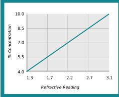
% Concentration = Refractive Reading x Refractive Factor Coolant Refractometer Factor % Brix = 3.2
