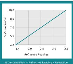
6 Concentration = Refractive Reading x Refractive Factor Coolant Refractometer Factor % Brix = 2.8
