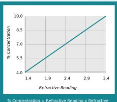
% Concentration = Refractive Reading x Refractive Factor Coolant Refractometer Factor % Brix = 2.9
